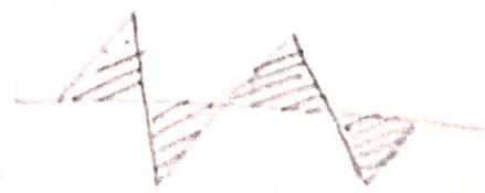
**Secondary Texture :** If the surface irregularities are of very longer wavelength ie two consecutive hills or two consecutive valleys one far apart it is created due to blunt tool, improper alignment of tool or workpiece.
