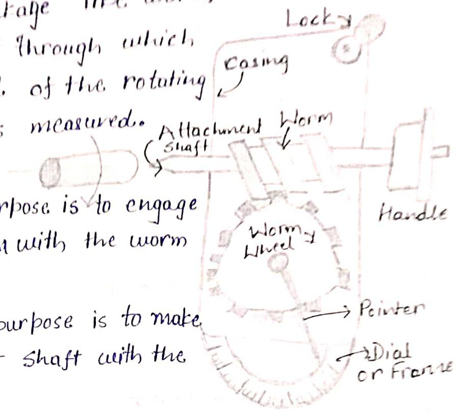
1. Lock; Its main purpose is to engage & disengage the worm with the worm wheel.
